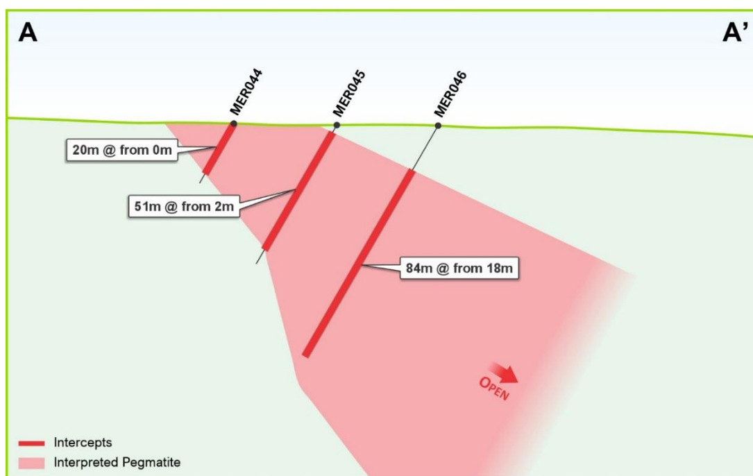
Figure 4: Cross section A–A' showing interpreted pegmatite geometry and selected drill intercepts
