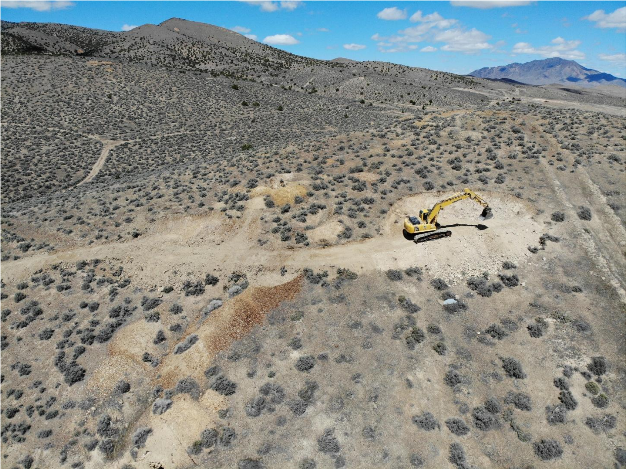
Figure 1. Drill pads being prepared at the historic Keystone Mine; part of WRX's larger flagship Keystone Polymetallic Project. Visible to the left of the excavator is the outcropping strike of the main Keystone vein trending off to the north and showing historic backfilled stoping to surface.
