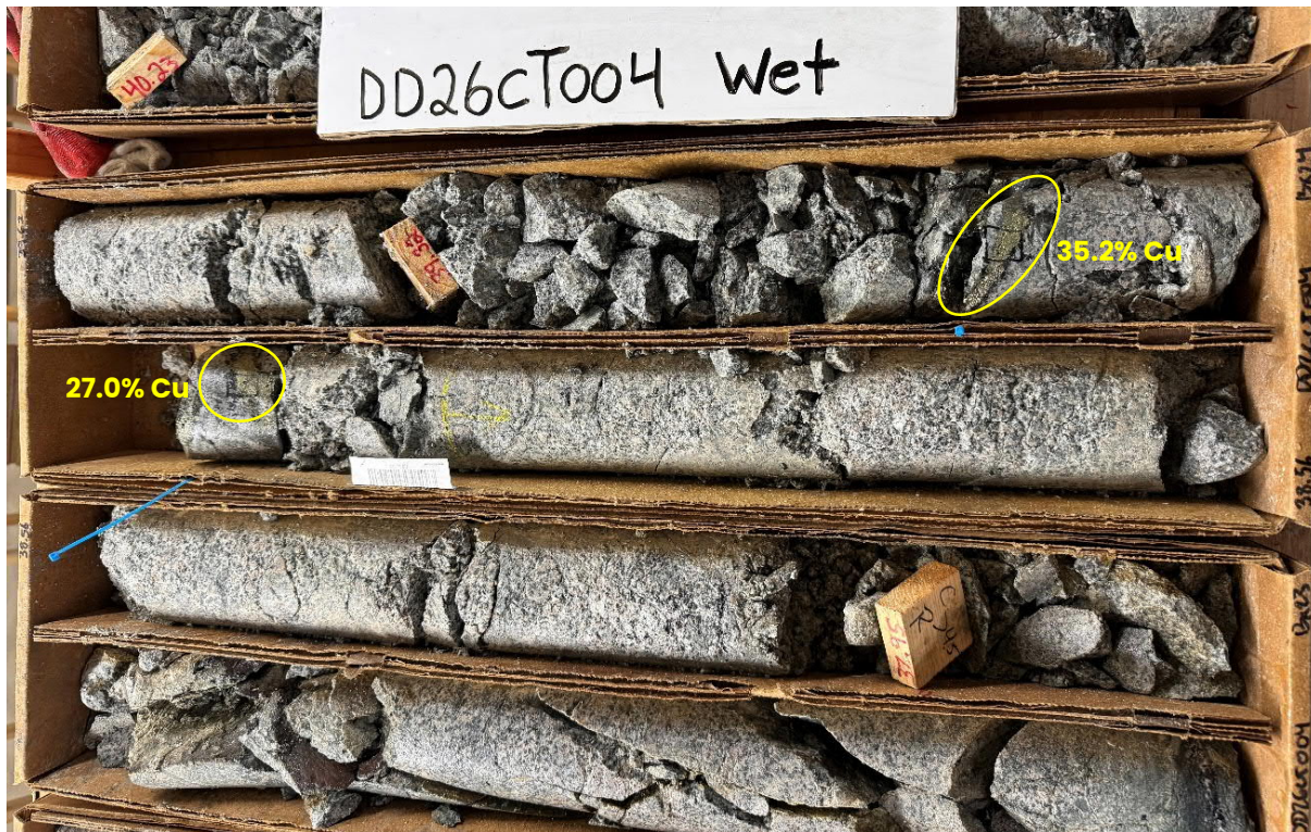
Figure 3: Chalcopyrite copper mineralisation and spot pXRF copper assays between 37.0–39.5m.
