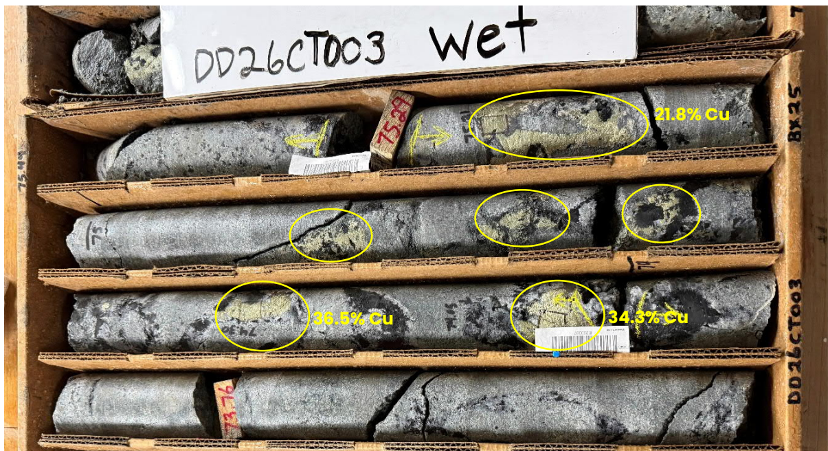
Figure 2: Visible chalcopyrite copper mineralisation between 74–76m down hole DD26CT003 with spot pXRF copper assays.
