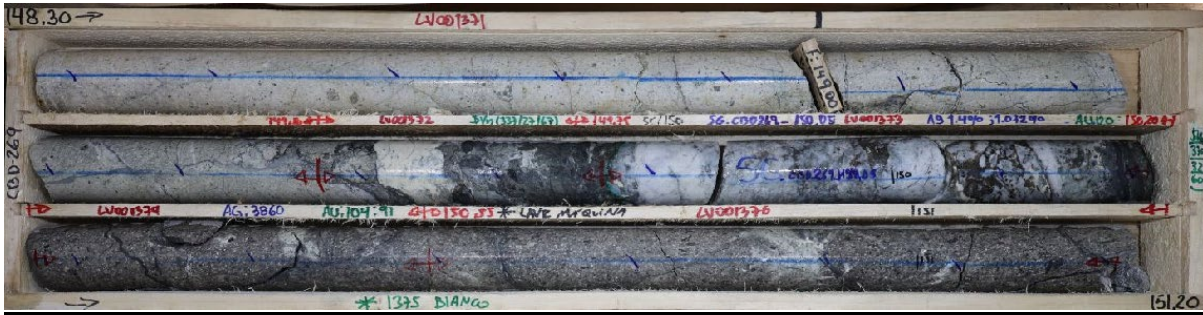
Figure 7. CBD269 Temer Main mineralised shoot quartz breccia, 0.8m @ 4,131g/t AgEq from 149.75m to 151m. Refer to Andean ASX release dated 2 December 2025.
