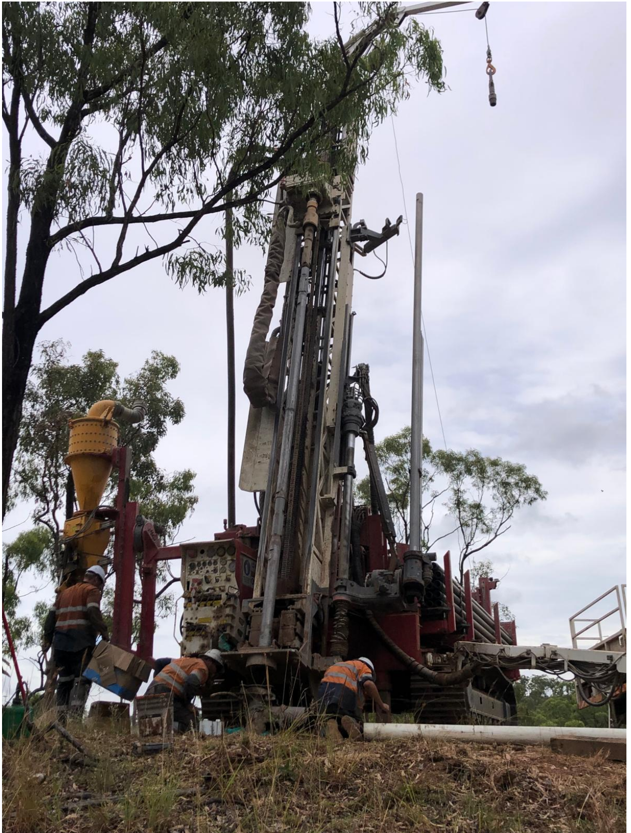
Figure 1: RC drill rig operating at the Clermont Gold Project.
