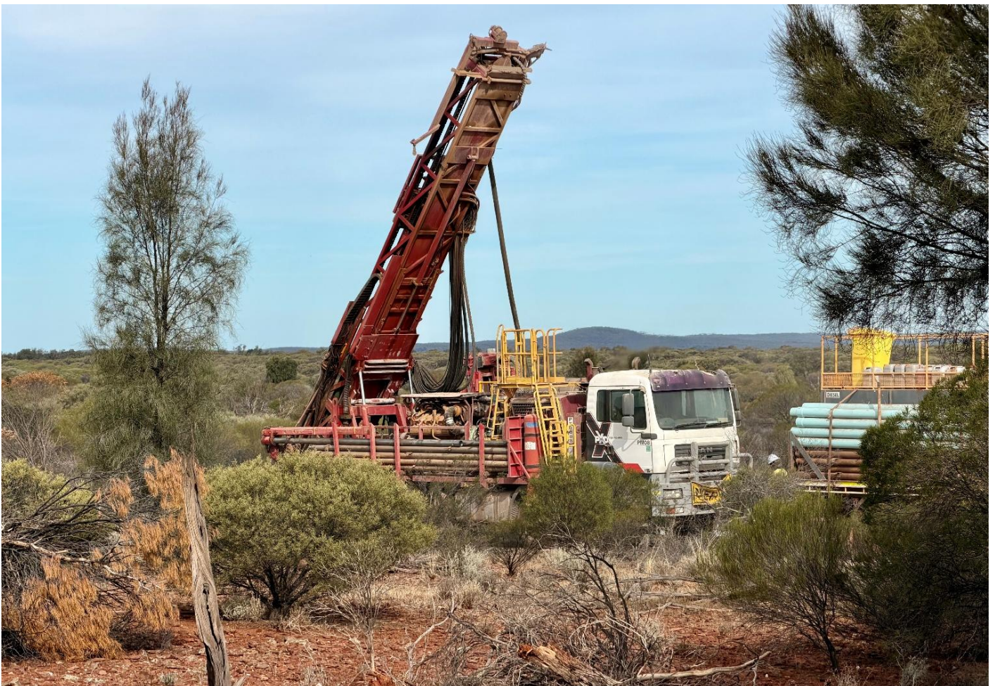
Figure 1: Image of the PXD RC rig drilling at Metzke's Find.
