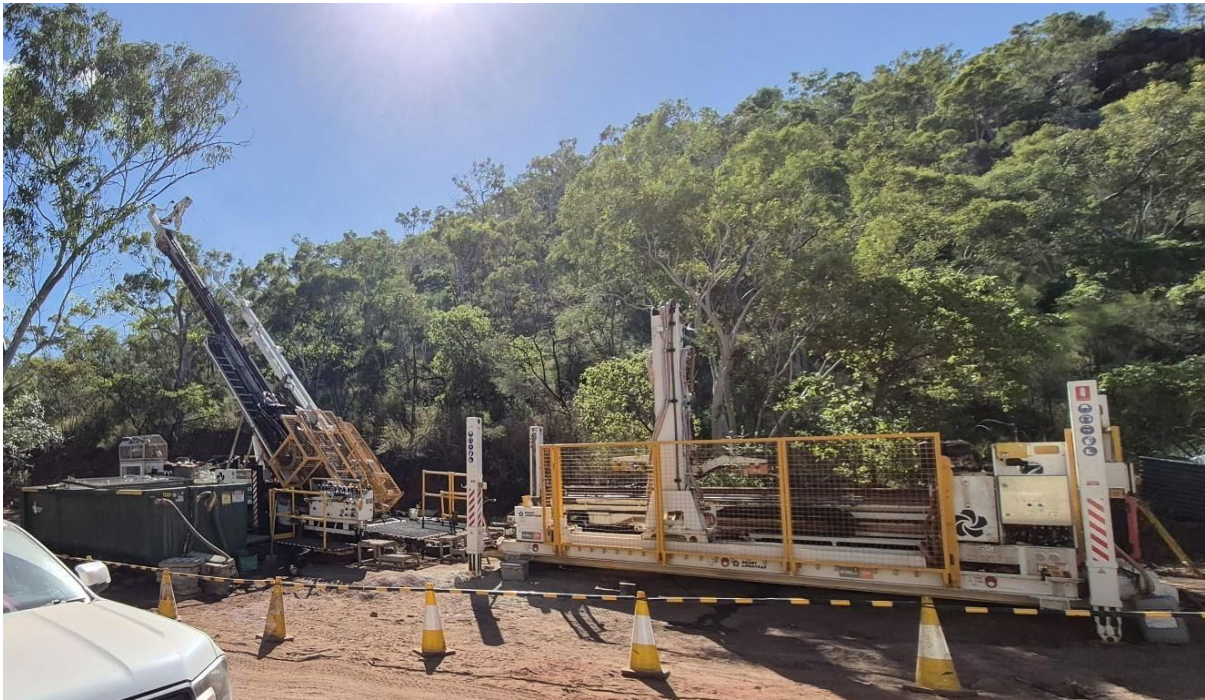
Figure 3. Diamond Drill rig operating at the Aquila Discovery, Mt Oxide Project
