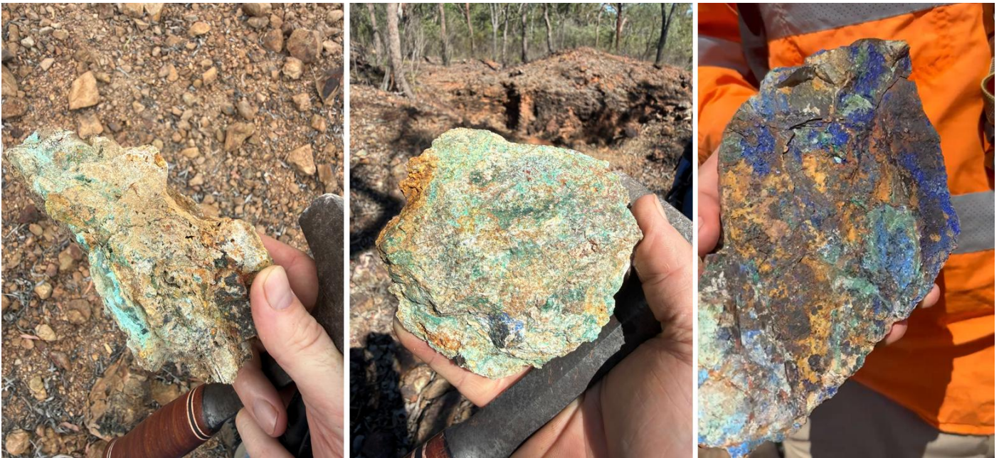
Figure 1 Examples of rocks from the Copper Hills mine dumps containing malachite and azurite (copper carbonate).
