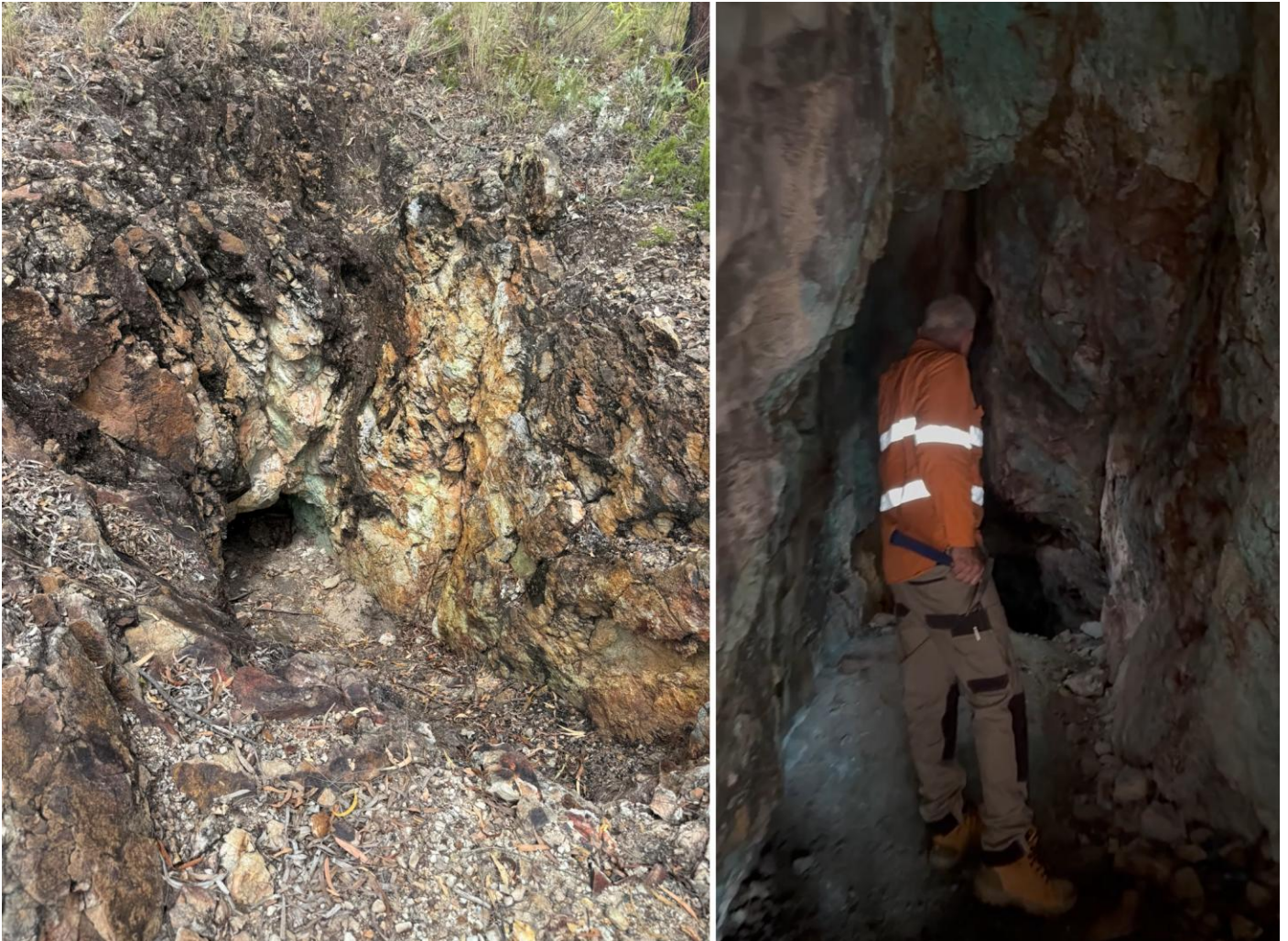
Figure 11 Left: Mine adit developed on a 1.5m wide vein with lesser stockwork and sheeted veins evident in selvedge of the mined out vein. Right: At the entrance of a mine adit developed on a 1m wide vein with malachite and azurite coating the mine walls and roof.
