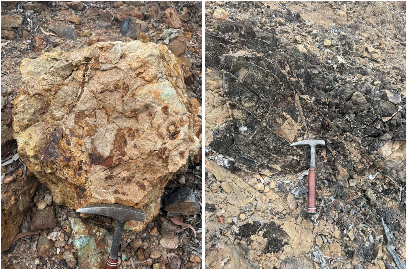
Figure 4 Examples of stockwork veins – Left: vein stockwork in a rock on the mine spoil dump. Right: Outcropping stockwork quartz veins outside of the historically mined vein.
