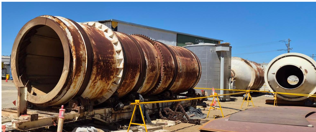
Figure 5: OzAurum agglomerator drum, cyanide tank, lime + cement silos at Polaris Engineering Services Henderson Facility
