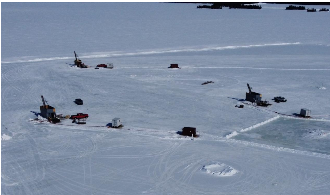
Figure 1: Three drill rigs completing the Golden Eye resource conversion program on the engineered ice pad (March 2026).
