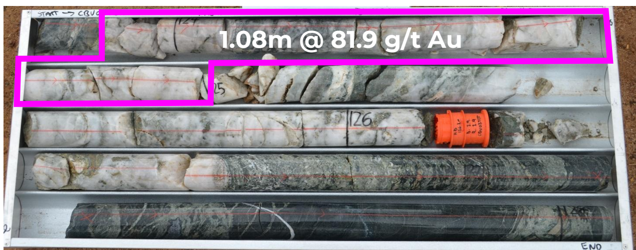
Figure 2: Typical vein-style high-grade gold mineralisation at Blue Vein, 1.08m @ 81.9 g/t Au from 123.92m (CBV037DT)
