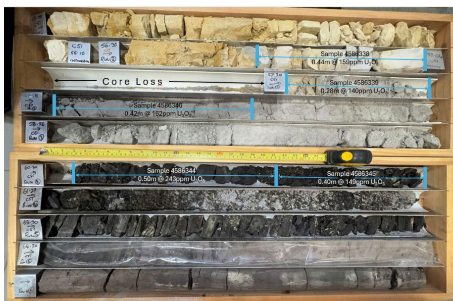
Figure 4 — Core hole C51, with significant uranium assay intersections marked. Note redox boundary becoming evident in the sample 4586338 sample interval.
