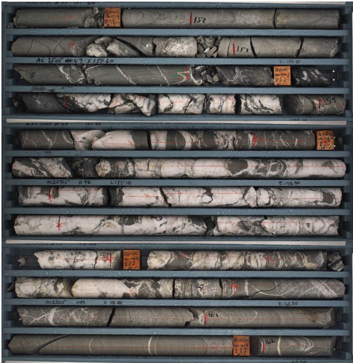
Figure 3: AC2505 Tray #47, #48, #49 (151.6m to 162.2m) showing styrolitic quartz
