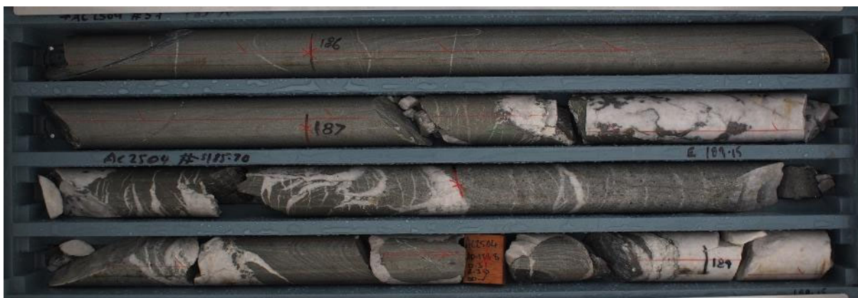
Figure 2: AC2504 Tray #57 (186m – 189m) with an example of tension vein array in sandstones and grits.
