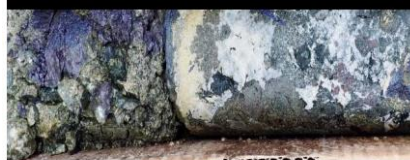
Bornite mineralisation in garnetiferous skarn, ZM17010, 179.4m
