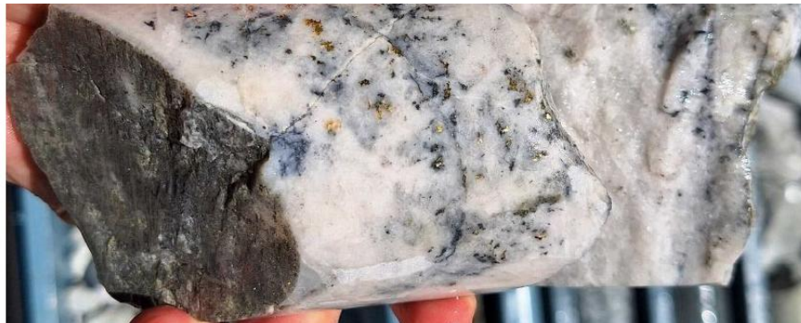
SDDSC161 intercept: 0.2 m @ 4,700 g/t Au and 0.26% Sb from 511.3 m showing abundant visible gold in a quartz-carbonate-stibnite vein. Part of a wider zone grading 3.4 m @ 466.4 g/t AuEq (466.0 g/t Au, 0.2% Sb) from 508.4 m. Core diameter is 63.5 mm.
