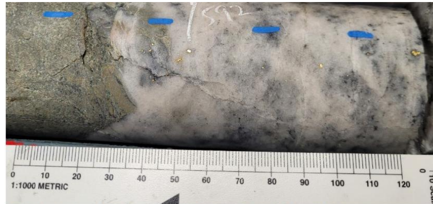
SDDSC082 4.3 m @ 72.6 g/t AuEq (71.5 g/t Au, 0.4% Sb) from 588.0 m showing uncut core with quartz-carbonate massive vein with visible gold. mm scale
