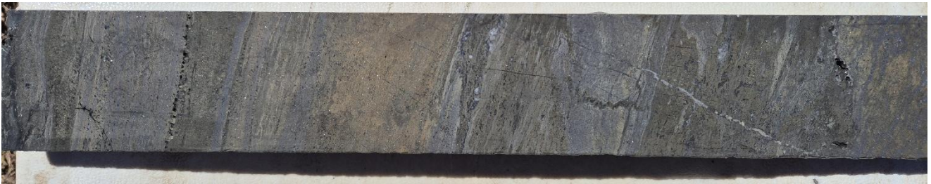
Figure 2: HQ3 drill core from hole CMKNI002 (Sample ID 162508), showing massive sulphide mineralisation, which returned 1.3m @ 5.4 g/t Au, 455 g/t Ag, 18.2% Zn, 7.8% Pb and 0.2% Cu .
