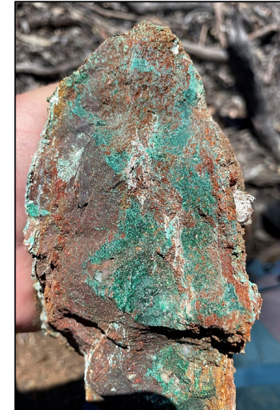
Copper smelter site, open cut workings and haematitic gossan with malachite (15.5% Cu, 0.42g/t Au, 29.1g/t Ag)
