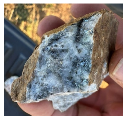
Quartz-carbonate vein breccia. Visible Stibnite. Sericite-quartz – mine dump (0.6% Sb, 0.08g/t Au, 994 ppm As)
