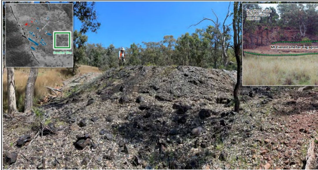
Copper smelter site, open cut workings and haematitic gossan with malachite (15.5% Cu, 0.42g/t Au, 29.1g/t Ag)
