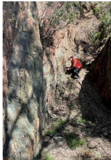
Copper smelter site, open cut workings and haematitic gossan with malachite (15.5% Cu, 0.42g/t Au, 29.1g/t Ag)
