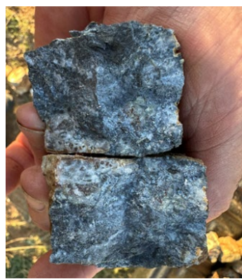
Quartz vein breccia with visible Stibnite – mine dump (5.75% Sb, 0.14g/t Au, 765 ppm As)
