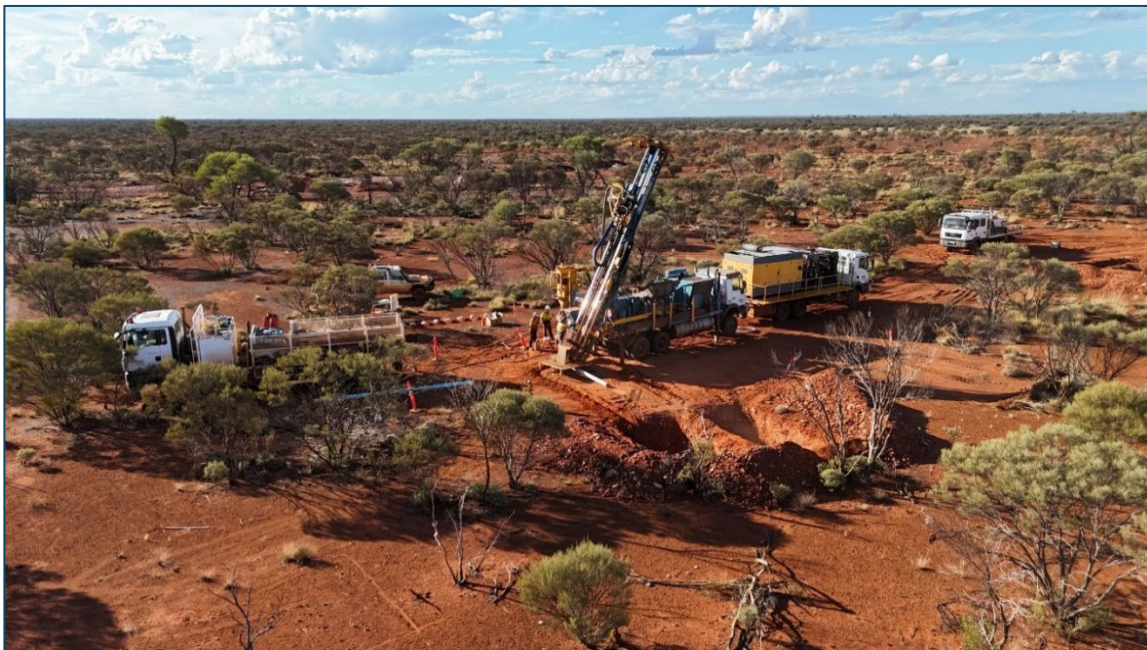
Figure 1: An aerial photo looking north over the RC rig that recently commenced extensional exploration drilling at the Arrakis gold discovery.
