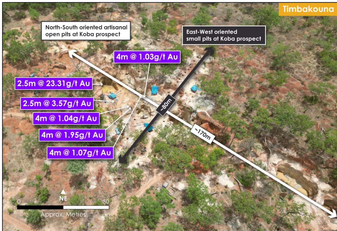
Figure 2: Artisanal workings at the Koba Prospect, Timbakouna, highlighted by north-south and crosscutting east-west structures with channel sampling from within artisanal workings producing gold grades of up to 2 m at 23.21g/t Au.
