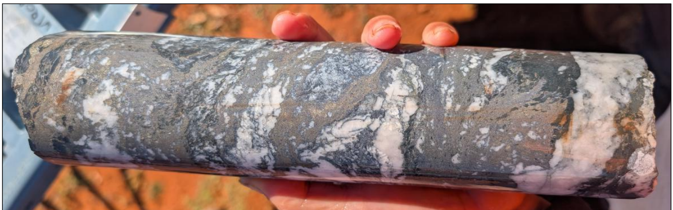
Figure 1 – Semi-massive/stringer sphalerite-galena-pyrite mineralisation @ 546.3m down-hole
