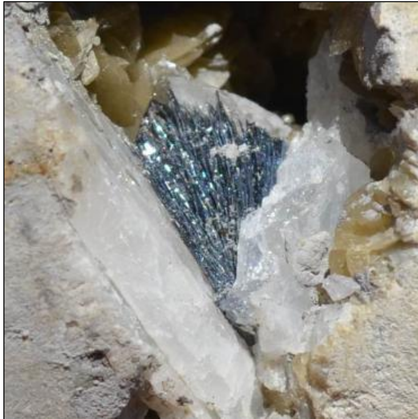
Figure 3: Stibnite (antimony sulphide) needles in fracture in core from BPD08. Antimony containing minerals at Bulla Park are tetrahedrite and stibnite
