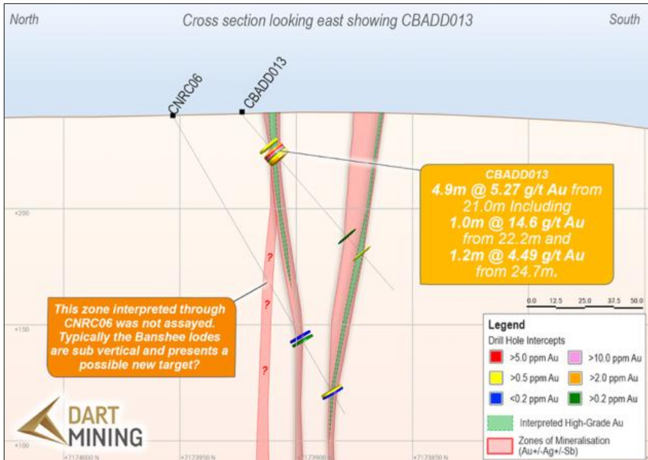
Figure 1: Cross section through CBADD013 showing gold assays and interpreted mineralised zones.
