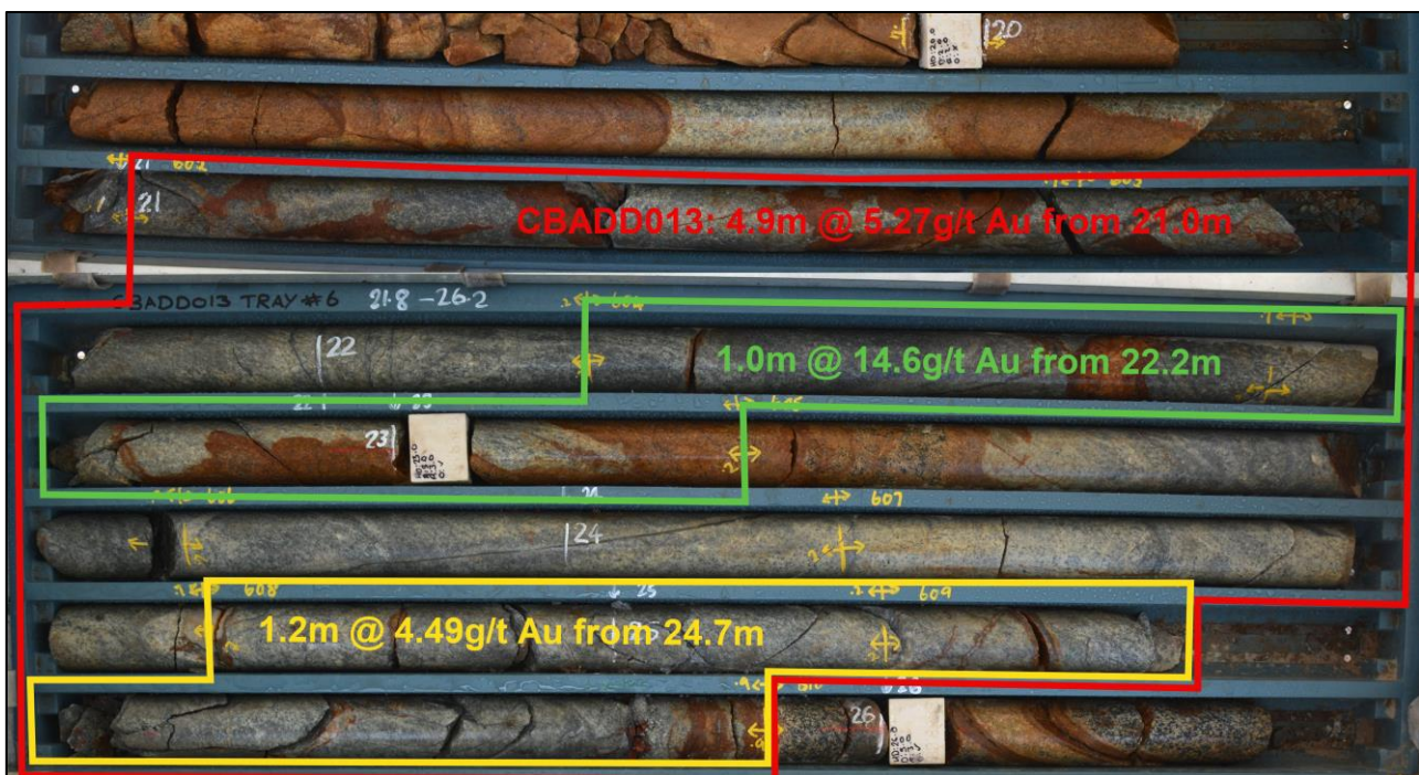
Figure 2: Core trays of CBADD013 highlighting the key thick gold zone and key assays intervals.
