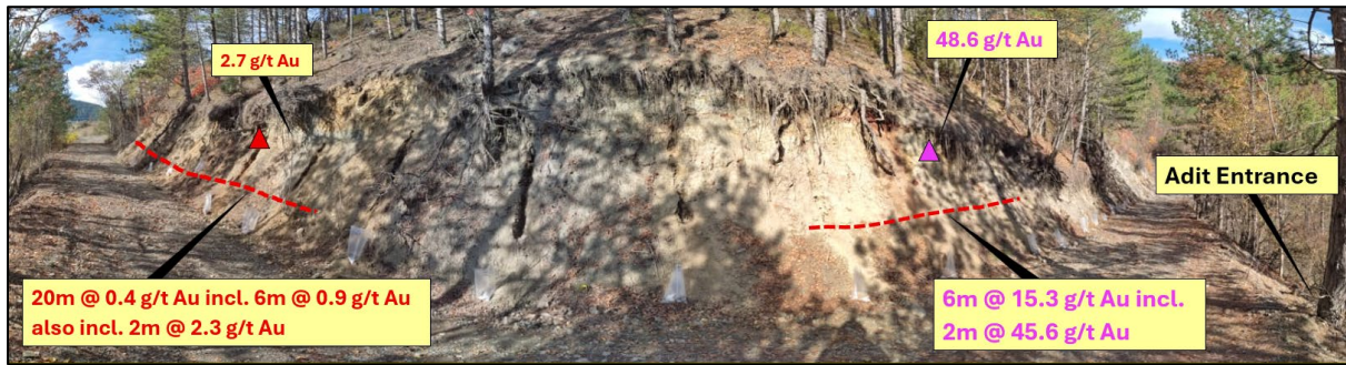
Figure 2. Mineralised outcrop at Drenjak showing channel and rock chip locations
