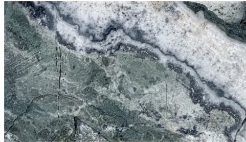
2 Ginguero banding in drill core from CDH-001 (3.00 m @34.7 g/t gold, 3,129 g/t silver from 111 m).
