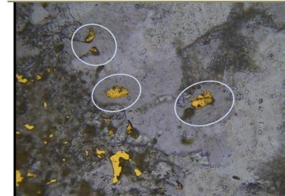
140002.13a. As above 600. \mu\text{m} ppl/rl. Free gold included in granoblastic quartz.
