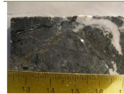
Left. 140002.08. Hydrothermal & tectonic overprinted, metamorphosed & metasomatised, sheared/fragmented dolerite
