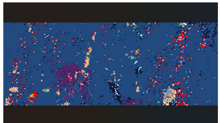
Figure 7: LIBS image (field of view ~5cm x 2cm) from CBDD011 ~295m showing coarse pyrochlores (red) in a matrix of dolomite (blue).
