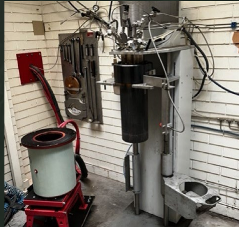
4Ltr pressure reactor and inductotherm heater
