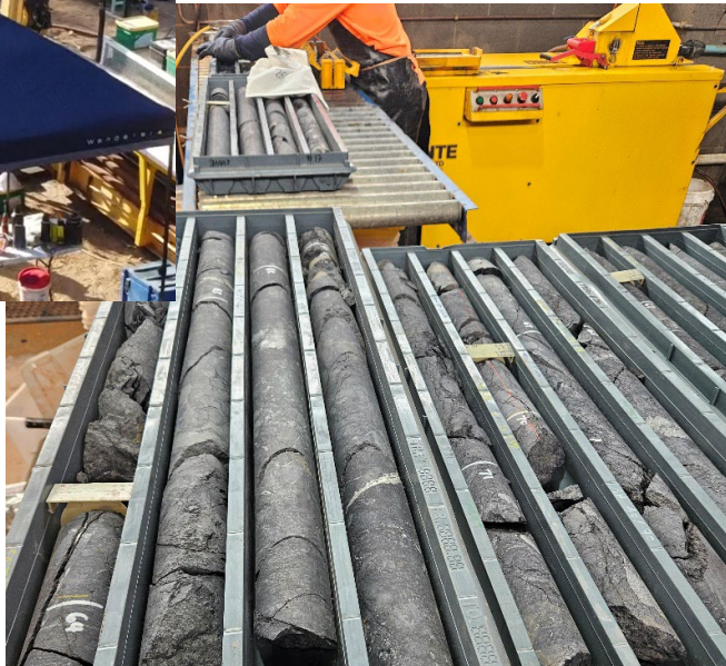
Right: SBD003 drill core about to enter the core saw at ALS preparation facility in Brisbane
