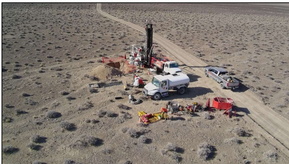
Figure 4. RC DRILL RIG ONSITE AT ALKALI FLATS
