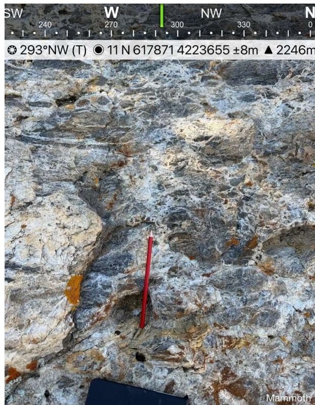
Figure 4 Close-up view of main fluor spar replacement body. The white material is fluor spar, and the grey material is fluor spar impregnated in limestone (pencil for scale)
