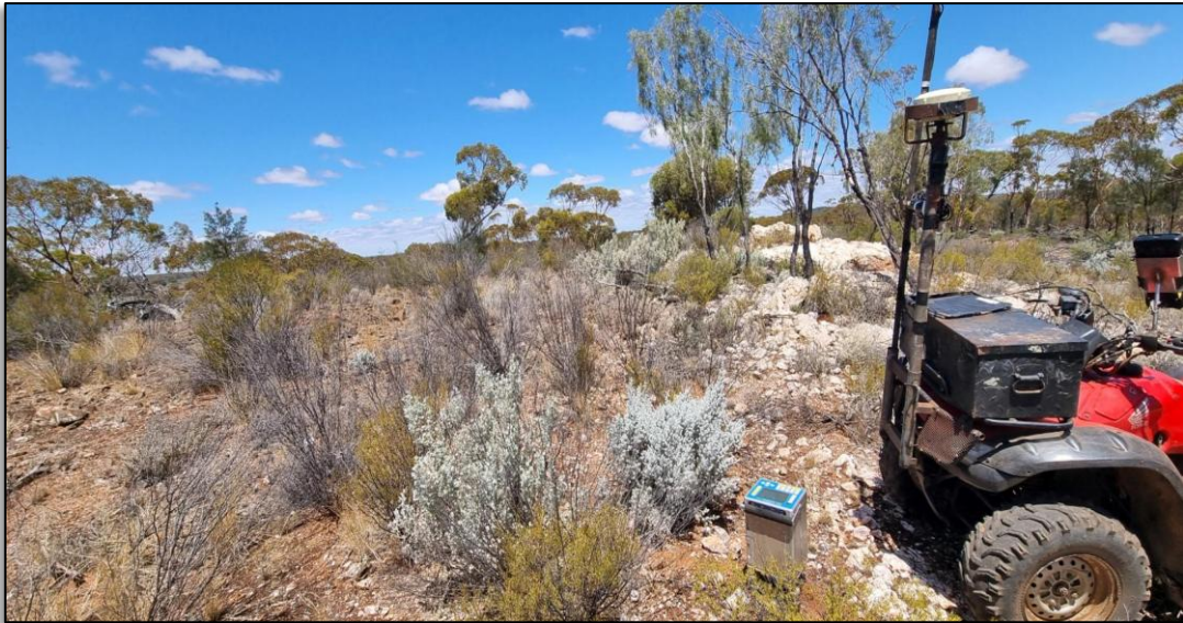
Figure 2: Ground gravity survey underway at the Mt Monger Gold Project, February 2026.
