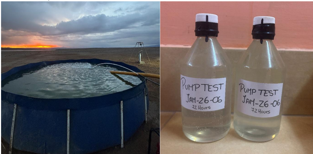
Figure 4. Pool being filled during pump test and sample bottles ready for assay with control marks.
