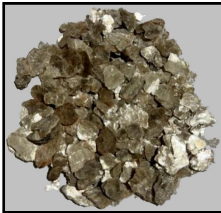
Figure 2: Mica portion produced after crushing to 8mm
