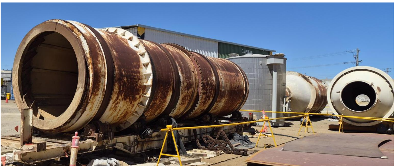
Figure 1: OzAurum agglomerator drum, cyanide tank, lime + cement silos at Polaris Engineering Services Henderson Facility
