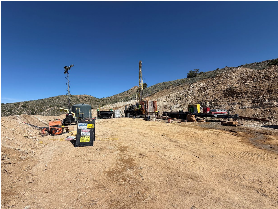
Figure 3: Dateline diamond drill rig testing the REE targets at Colosseum
