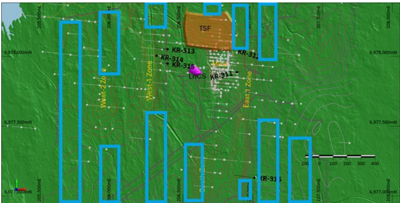
Drill hole location map showing the holes KR-311 to KR-316. Holes KR-311 and KR-312 targeted near-mine mineralisation, while KR-313, KR-314 and KR-315 tested the mineralised zone west of the mine known as West-1. Hole KR-316 was more exploratory, targeting a gravity and passive seismic anomaly south of the mine. Blue polygons are seven known exploration target parallel zones open to the north and south. The current iteration of the Exploration Target currently being revised
