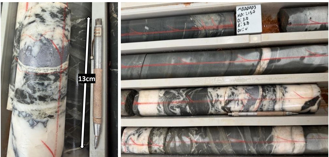
Photo 1 & 2: Hydrothermal alteration & quartz veining with massive galena (lead) bleb with trace pyrite (MBDD003; 216m).
