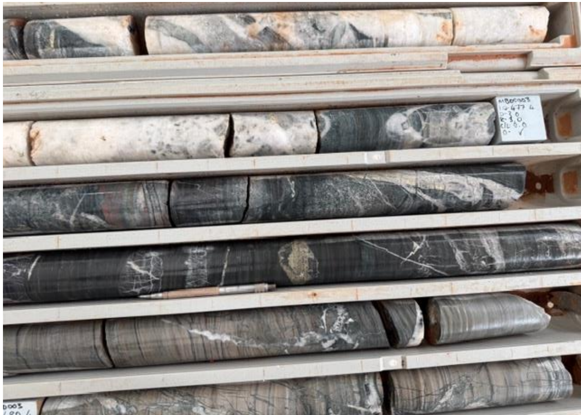
Photo 8: Quartz veining & hydrothermal alteration with layers of magnetite & disseminated & veinlets of pyrite (MBDD003; 476 – 480m).
