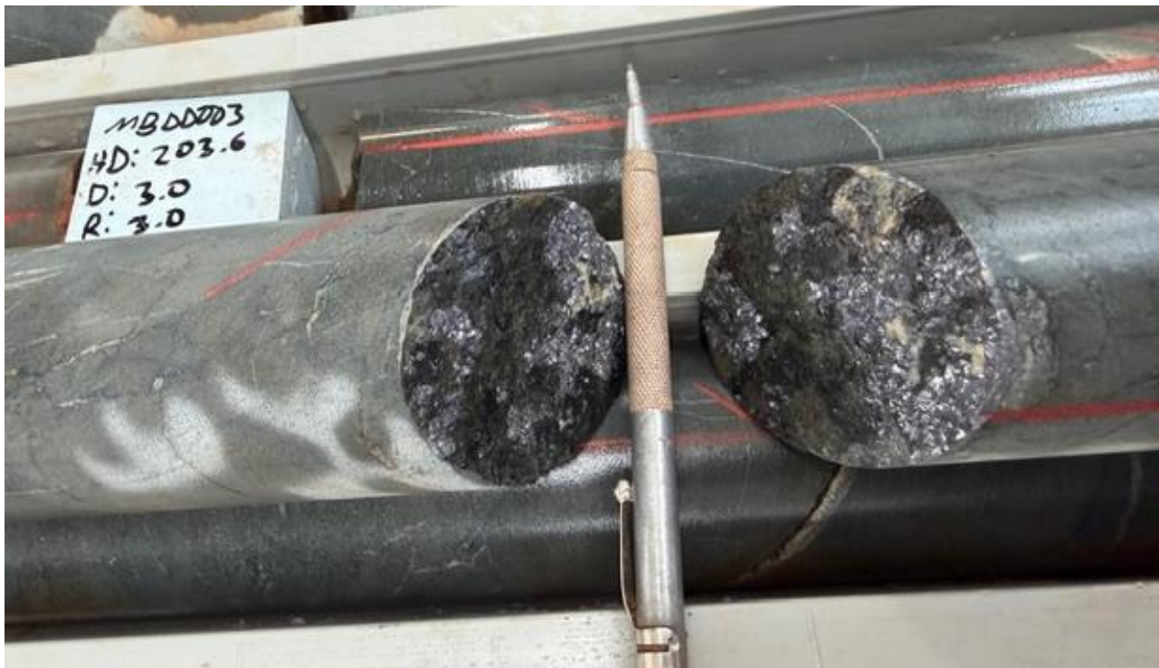
Photo 3: Galena, a lead sulphide mineral, on core fractures in hydrothermally altered siltstone unit (MBDD003; approx. 204m).
