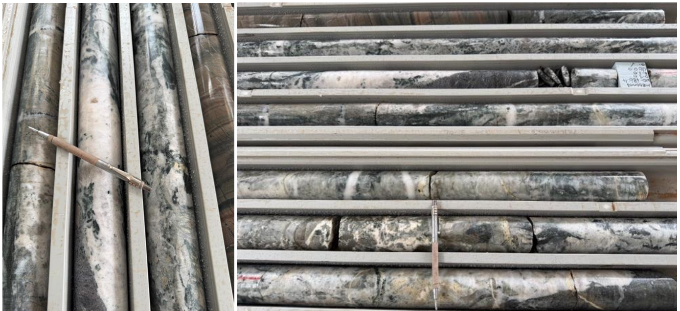
Photo 6 & 7: Quartz veining and hydrothermal alteration with blebby galena (lead) and pyrite (MBDD003; 484 - 490m).
