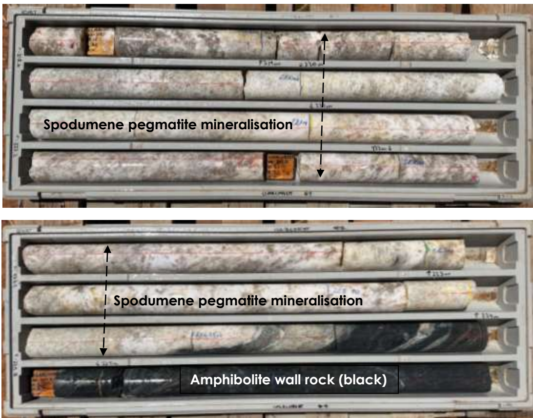
Photos 1 and 2. Coarse-grained spodumene in diamond drill core from CLMRC055DT from 220m to 224.35 with an average grade of 1.33% Li 2 O and 74ppm Ta compared to the amphibolite wall rock.
