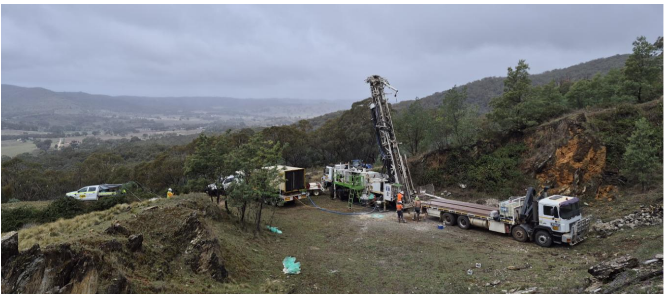
Figure 1: Photo of reverse circulation drill rig on site and drilling at Lewis Ponds
