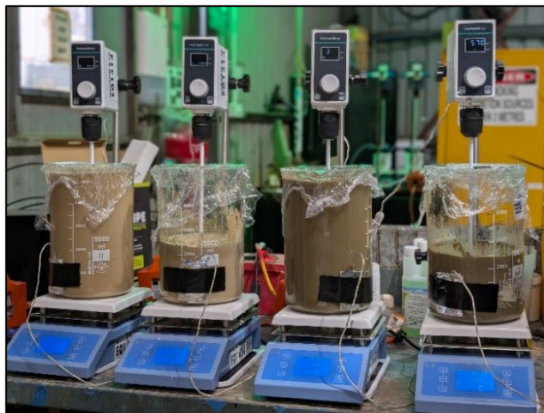
Figure 2: Stirred vessel leach apparatus
