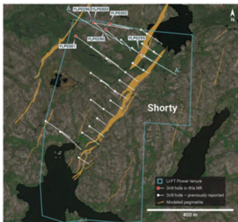
Figure 22: Plan map showing Shorty tenure boundary, pegmatite dykes, 2023-2024 drill traces, and the 2025 resource delineation holes.
