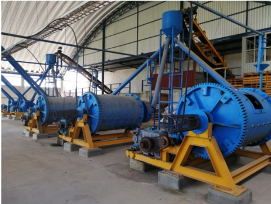
Figure 1: Tecomatlán Plant – Ball Mills
