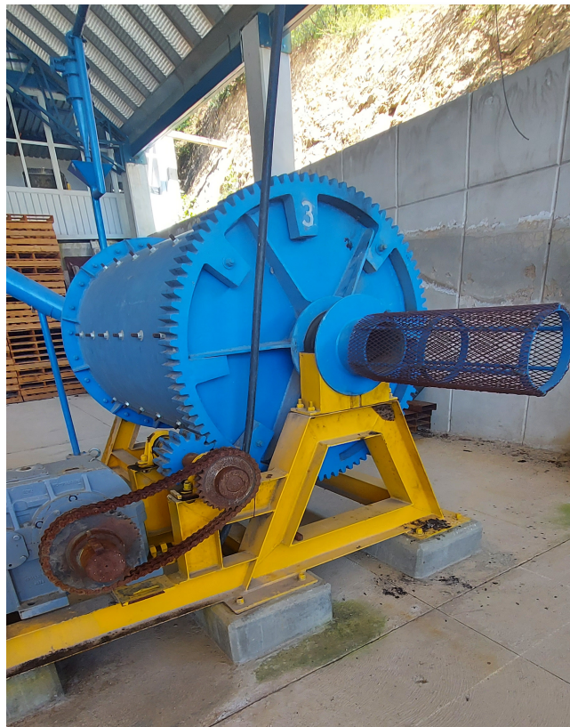
Figure 2: Tecomatlán Plant – Ball Mill #1
