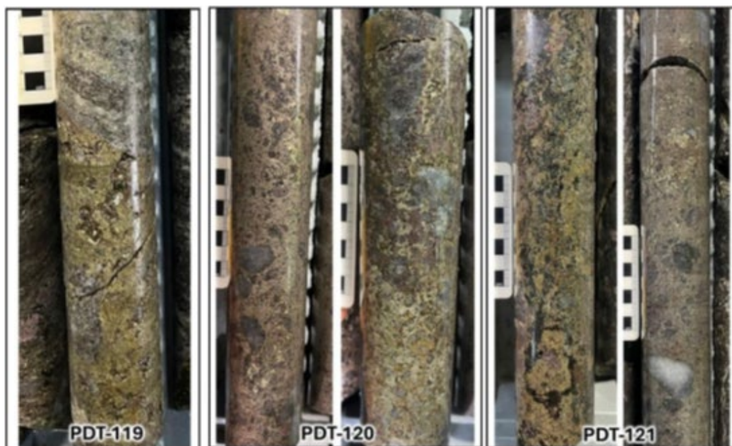
Figure 6: Mineralised intervals at Touro Prospect drilling. From left to right: PDT-119 from 65.5m downhole. PDT-120 from 66.25m (visual estimate of 8% chalcopyrite and 12% sphalerite) and 69.2m (visual estimate of 1% chalcopyrite and 25% sphalerite). PDT-121 from 95m and 101.85m (Visual estimate of 3% chalcopyrite + 1% sphalerite, and 10% chalcopyrite + 5% sphalerite, respectively). Depth refers to base of core in photo. Dark brown mineral is sphalerite (zinc sulphide), golden colour is chalcopyrite (copper sulphide), pale yellow is pyrite (iron sulphide) and bronze colour is pyrrhotite (iron sulphide).
