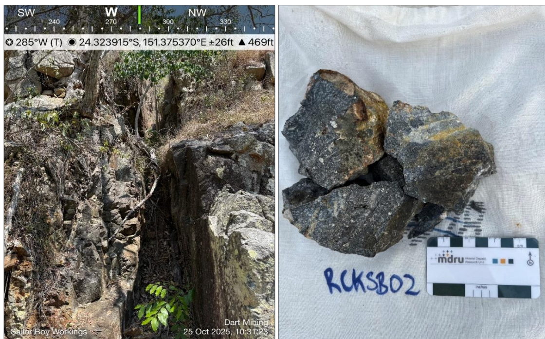
Figure 5: Sailor Boy workings from base of creek bed (left). High grade sulphide mineralisation present in the wall rock (right) assays 8.97g/t Au and 13.45g/t Ag (RCKSB02).
