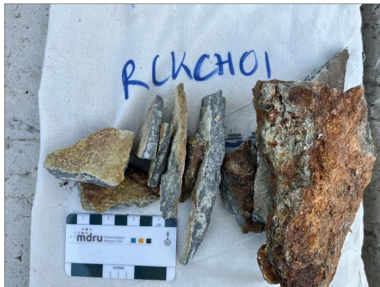
Figure 4: Chandlers composite sample from vein outcrop which assayed 109g/t Au and 105g/t Ag (RCKCH01).
