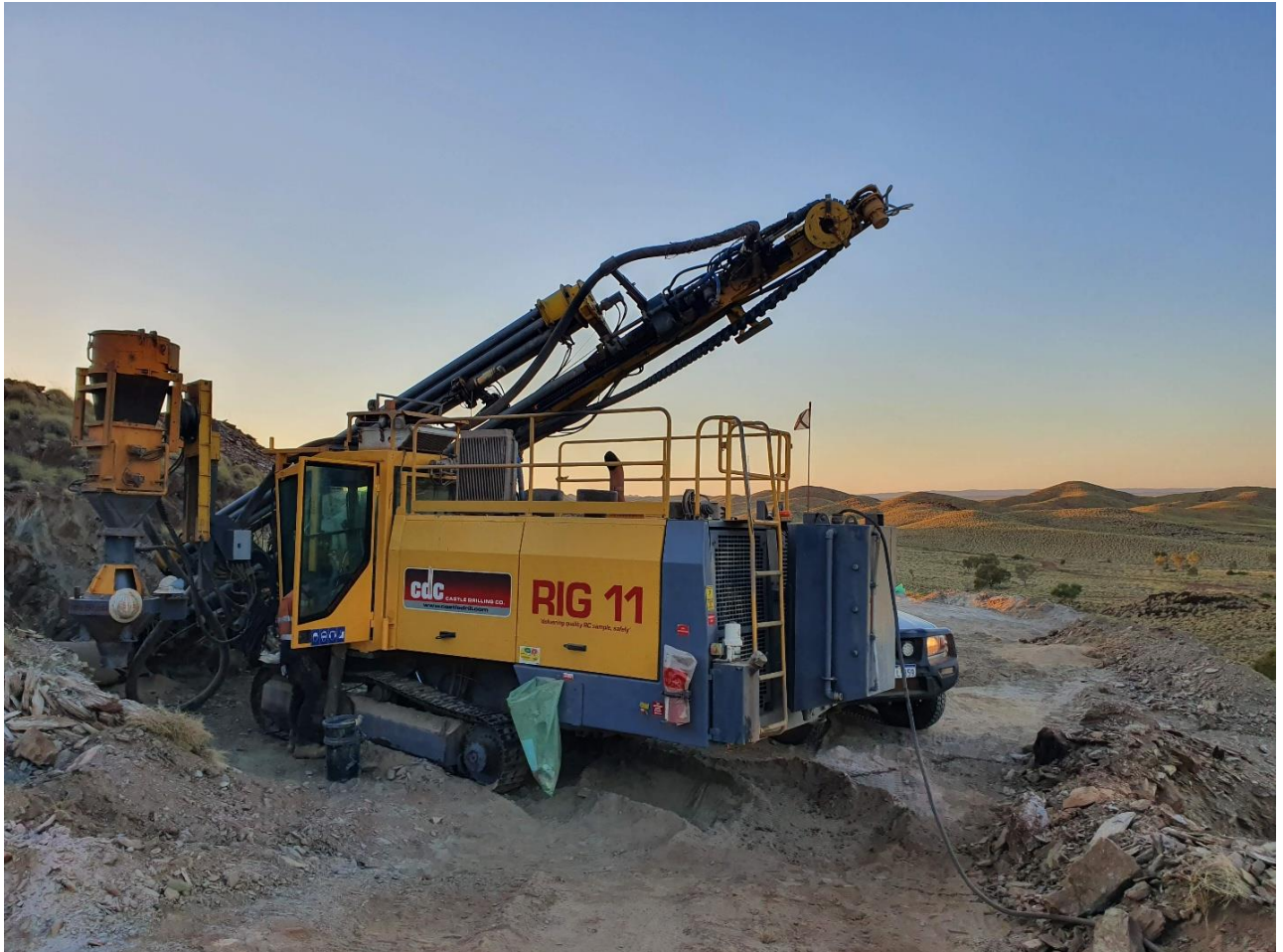
Figure 10: Specialised track mounted drill rig to be used in the upcoming RC program.
