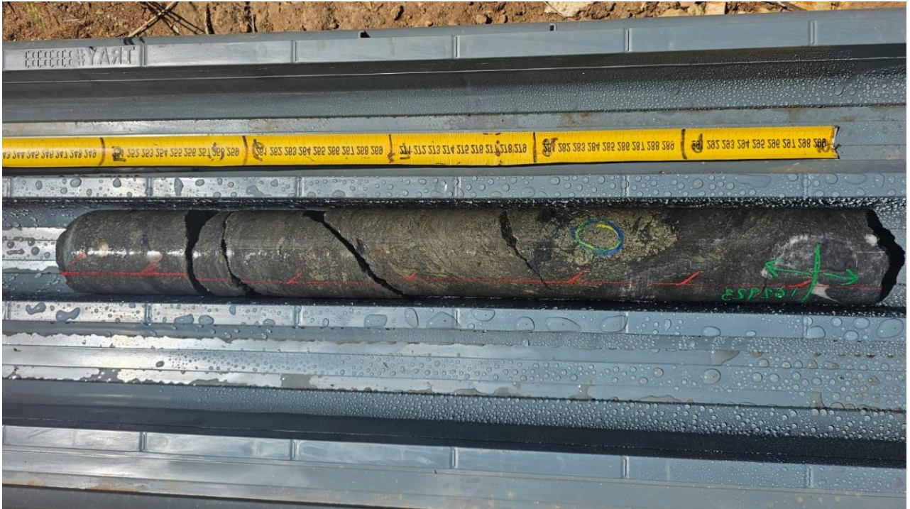
Figure 2: Diamond drill core (HQ) from hole CMKNI004 from 230.4m to 230.9m, showing a ~50cm massive sulphide vein comprising approximately 85% pyrite, arsenopyrite and proustite, hosted within sheared rhyolite porphyry.
