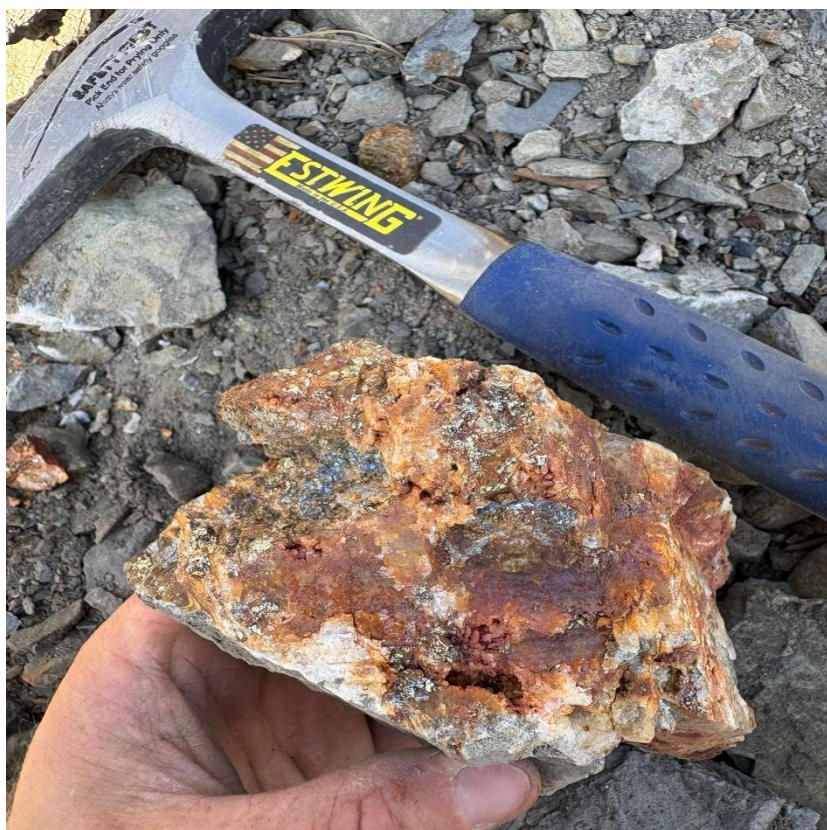
Figure 2: Rock Sample GR019 from Davis Mine prospect – Grading 1.96% Cu, 1.465% Zn 0.29% Pb
