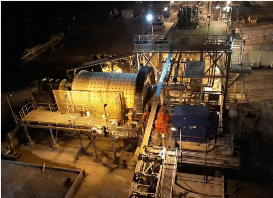
Figure A16: Existing 1800kW Ball Mill
