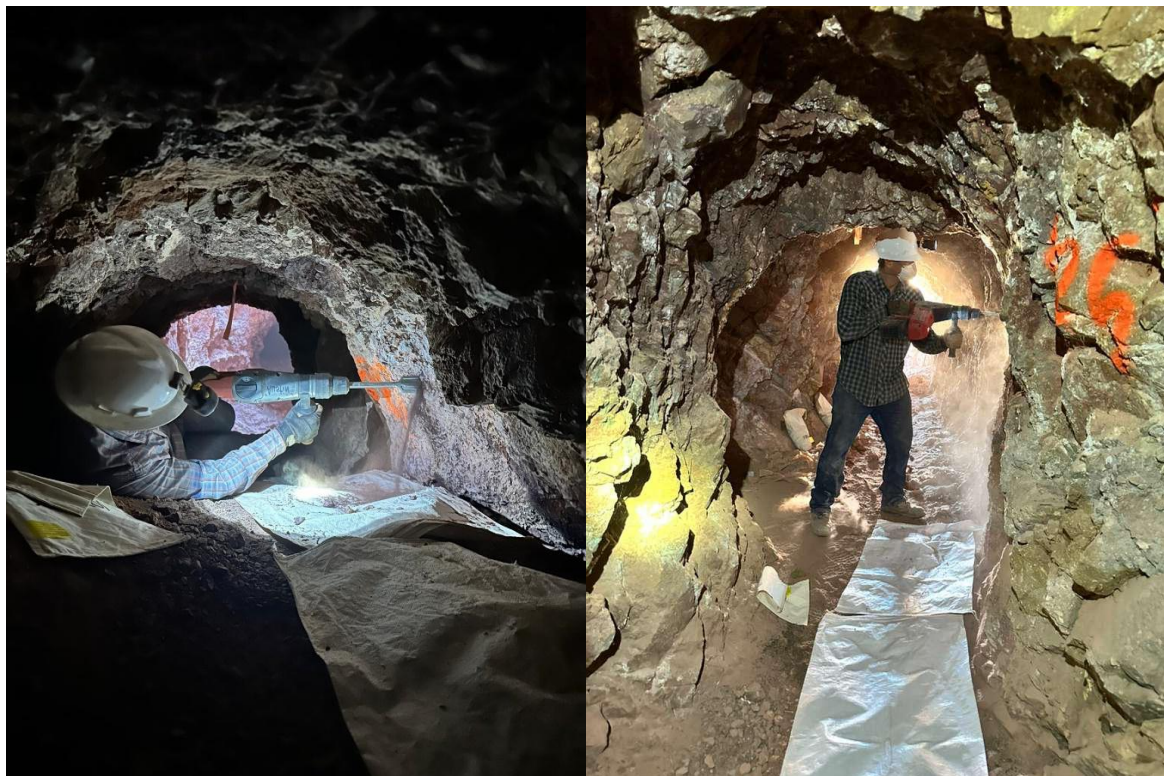
Figure 3. Underground chip-channel sampling with demolition hammer and chisel bit at Red Bird.
