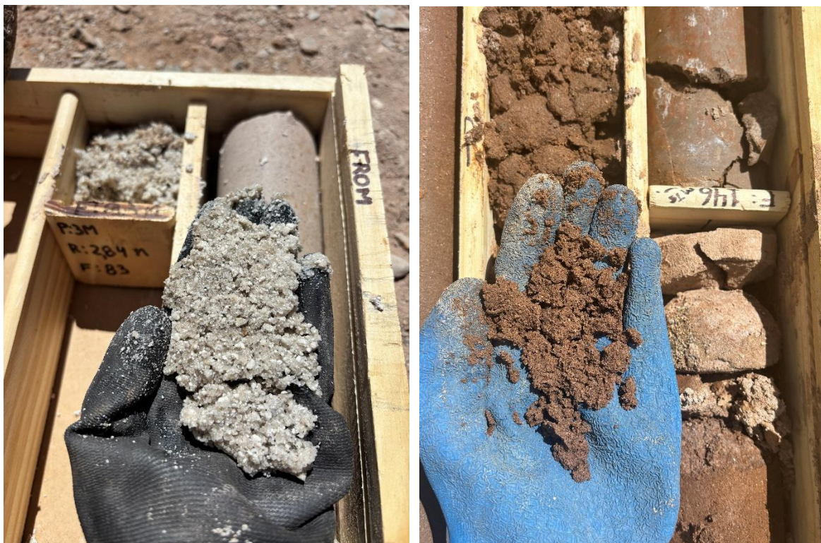
Figure 2. Core showing sandy sequences left at 284m depth and right at 146m depth that were recorded at a 1,200L/hour pump rate.
