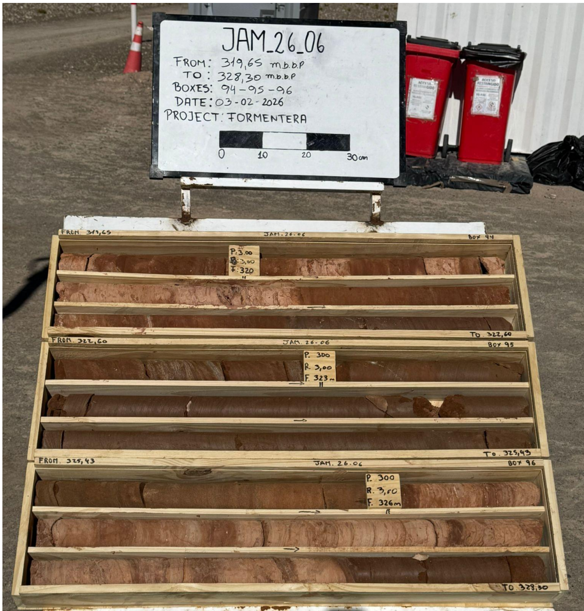
Figure 4. Drill core showing changes in lithology from sandy to silt to gypsum to carbonates within 3m.
